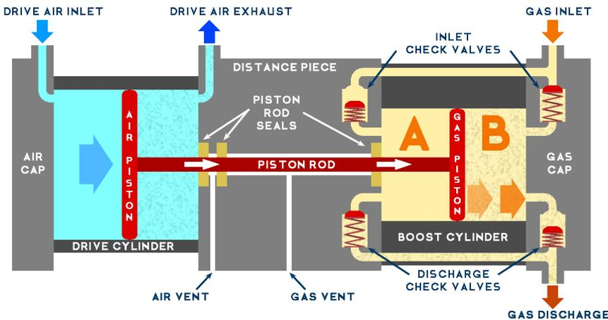
The pistons are traveling to the right and compressing the gas in chamber "B" while pulling gas into chamber "A".
