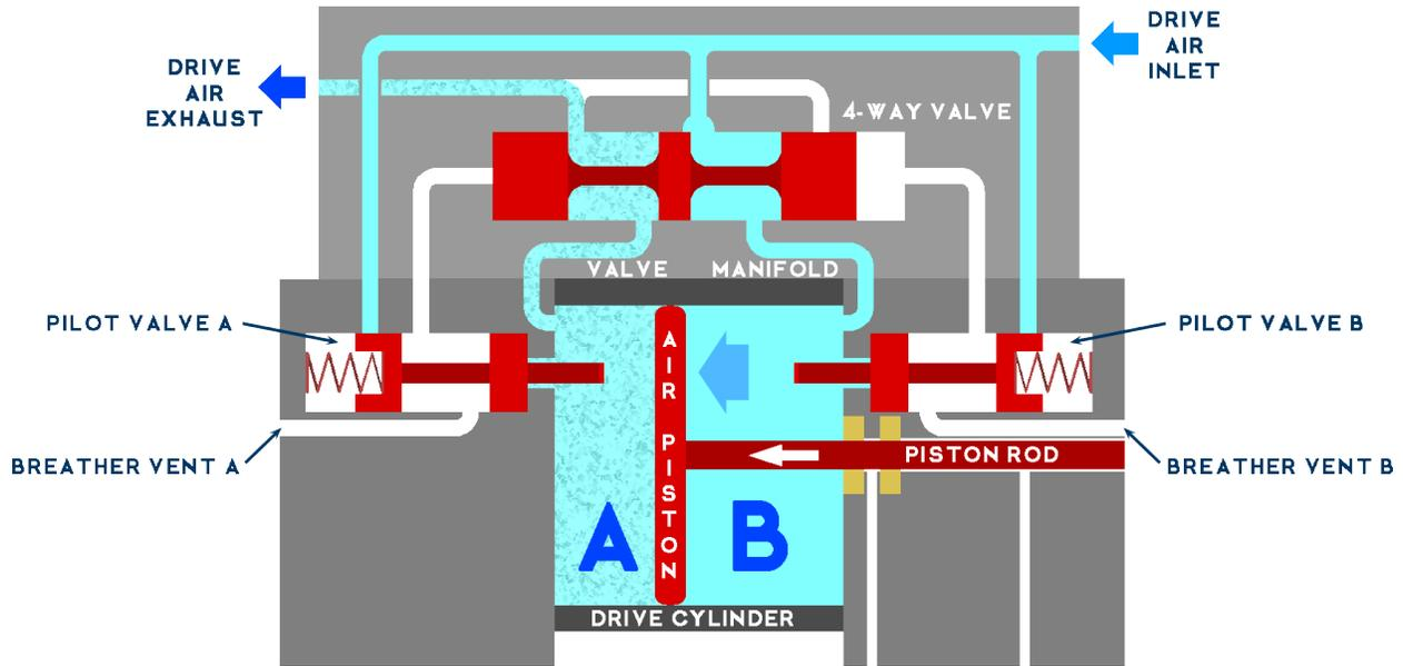
In the sketch below, the air piston has reached the end of its stroke and opened pilot valve “A”. This closes breather vent “A” and sends pilot air to the left pilot port on the 4-way valve. The 4-way valve shifts to the right, opens chamber “B” to exhaust and supplies drive air to chamber “A”. The air piston moves to the
